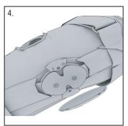
4. Install the extension stop (E) on the extension stop side of the hinge, and the flextion stop (F) on the flexion stop side of the hinge. The stops for both hinges must be set to the same settings.
