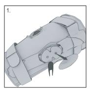
To remove the hinge cover cap, insert the provided tool into the space in the back of the hinge. The cap will come off using a twist or pry motion.
